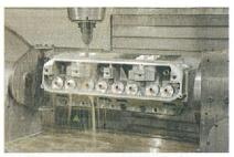
Since Indy Cylinder Head performs all the finish machining and final CNC work on their raw cylinder head castings, their 440 EZ heads are available in a variety of configurations. Variations include the "as-cast" 270cc with standard port window, the partially CNC-ported 275cc Max Wedge EZ-1, the fully CNC-ported 295cc Max Wedge Little EZ, and the fully CNCported 325cc offset rocker Max Wedge Big Easy.
