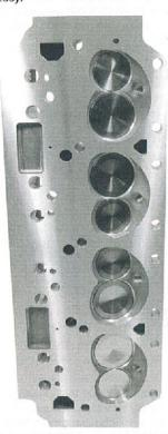
For our low-deck 500-cube aluminum street wedge's goals of street torque and moderate rpm, Indy went with the 275cc EZ-1. These heads feature CNC profiling of the port window to Max Wedge dimensions, as well as CNC porting in the allimportant bowl area.
