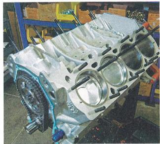
The assembly of our aluminum Maxx block bottom end was detailed in the May issue of *PHR*. In preparation for installing the Indy EZ-1 cylinder heads, the decks received a set of ARP studs. With a 0.039-inch Fel-Pro 1009 gasket and the full-dished Diamond pistons, the compression ratio works out to a pump gas—friendly 10:1.
