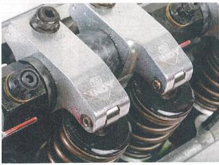
With the T&D 1.6:1 ratio rockers the custom COMP solid-lifter camshaft (grind number CRB3-6579-6583-S108) delivers a gross valve spec of .594/.612 inch. The valve lash was set to .018 inch (hot) on both the intake and exhaust.
