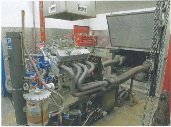
Bolted to the Indy SuperFlow dyno, the aluminum wedge was able to prove its capabilities. Tested at an acceleration rate of 600 rpm per second, the street combo delivered 662 lb-ft of torque at 4,500 rpm, with 657 peak horsepower on tap at 6,100 rpm.
