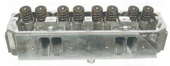
Viewed from the intake port side, the large port window and CNC work to the intake port entrance is readily apparent. The heads were set up by Indy with a COMP spring package compatible with a solid flat-tappet camshaft using a dual spring assembly, steel retainers, and 10-degree locks.
