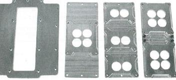
The flexible Mod Man intake allows a broad range of popular induction options simply by replacing the top plate. Top plates include a blower mount, single four-barrel, Six Pack three two barrels, or the dual quad top used in our application.
