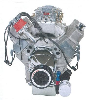
Fully assembled and ready for the dyno, Indy's dual-quad aluminum wedge was nothing short of a thing of beauty. For dyno trials, the engine would be fitted with a Meziere electric water pump and a set of 21/8-inch dyno headers. We may be restricted in our choice of headers with the Valiant; a set of custom units may be our best choice to fit in the A-Body's chassis.
