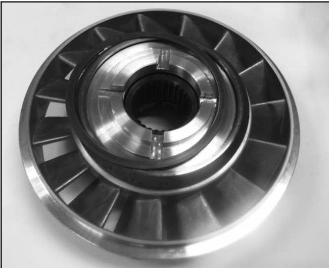
STEP 7 - Flip the stator over and remove the snap-ring holding the "A" side aluminum stator cap in place. Set the stator cap and snap ring to the side.
