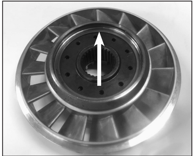
STEP 8 - DO NOT remove the second snap ring under the "A" stator cap as indicated by the arrow.
