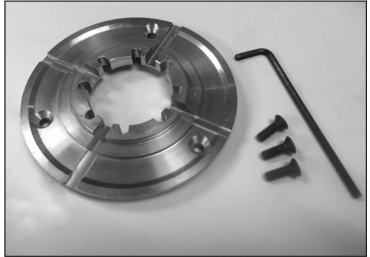
STEP 6 - Using a 1/8" allen key or socket, remove the (3) 10-32 x 5/8" allen head screws from the aluminum stator cap on the "B" side of the stator. Remove the cap itself. You may need to use an impact-type screw driver with an 1/8" allen bit. Place the "B" side aluminum cap to the side.
