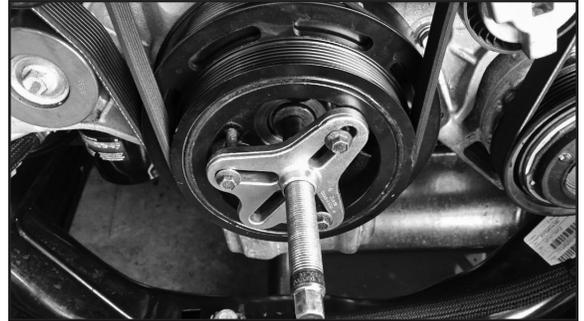
The OEM crankshaft does not have a keyway. The ATI Super Damper comes with a keyway and ATI offers a Drill Pin Fixture Kit (#918008-1) to install a pin to engage the keyway. ATI highly recommends pinning the crank. With boost, there is added resistance and the pin is necessary to prevent the damper hub from spinning on the crank snout. **There is NO warranty on cracked, spun or damaged hubs if the pin kit is not used!**
