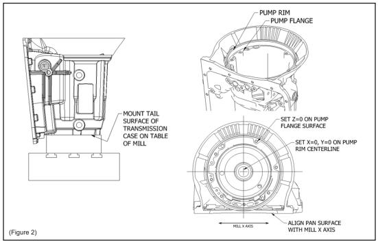
Step 3. Machine the front of the case
