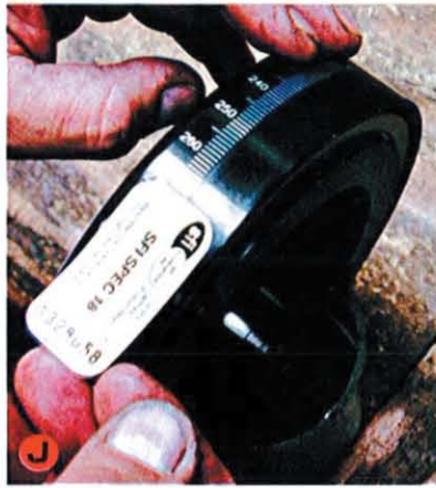
A new SFI-approved sticker is installed, and corresponding serial number is stamped on the outer shell. The unit is boxed and returned to the customer in as-good-as-new condition.
